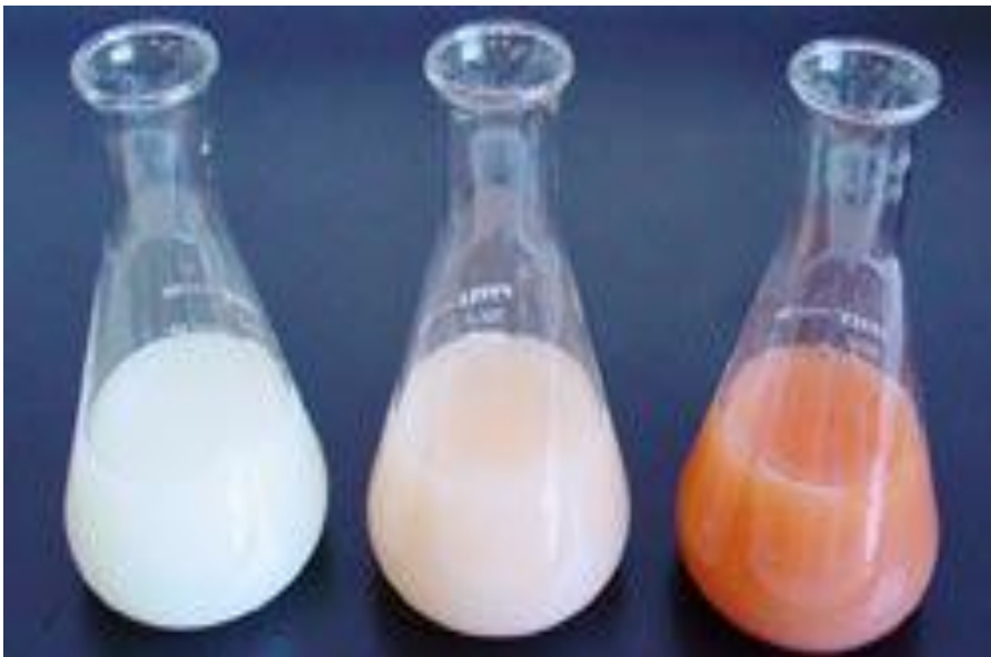
Figure 2 : Left flask: before the titration endpoint, addition of \text{Ag}^+ ions leads to formation of silver chloride precipitate, making the solution cloudy. The chromate indicator gives a faint lemon-yellow colour. Centre flask: at the endpoint, all the \text{Cl}^- ions have precipitated. The slightest excess of \text{Ag}^+ precipitates with the chromate indicator giving a slight red-brown colouration. Right flask: If addition of \text{Ag}^+ is continued past the endpoint, further silver chromate precipitate is formed and a stronger red-brown colour results. NB: The titration should be stopped when the first trace of red-brown colour is observed. Using an incompletely titrated reference flask for comparison is a helpful way to identify the first appearance of red-brown colouration.
