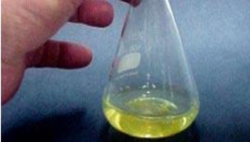
Figure 1 : Before the addition of any silver nitrate the chromate indicator gives the clear solution a lemon-yellow colour.
